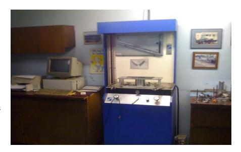
The design testing was much simpler. The runner lengths were measured from the outside of the head flange to the top most part of the runner or velocity stack. The Plenum volume was checked by sealing off the throttle body flange, and filling the plenum with fluid from the head flange. The manifold was filled up to the start of the runners. I also added some additional comments to a few manifolds for things that I noticed during testing.
